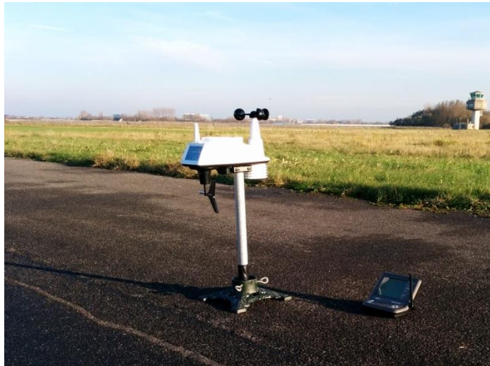
Figure 43: Davis weather monitoring system
