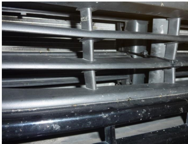
Figure 46: Active grill vanes in open position
