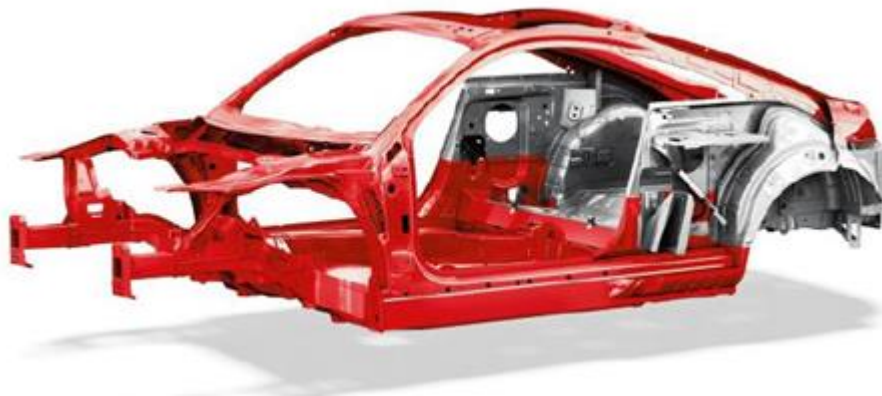
Figure 5-3: Hybrid steel-aluminium body construction of the 2006 Audi TT. (Source: European Aluminium Association, 2013a)
