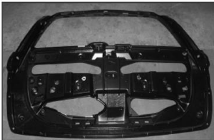
Figure 5-5: 2009 Lincoln MKT die cast magnesium tailgate inner panel. (Source: Gibbs, 2010)
