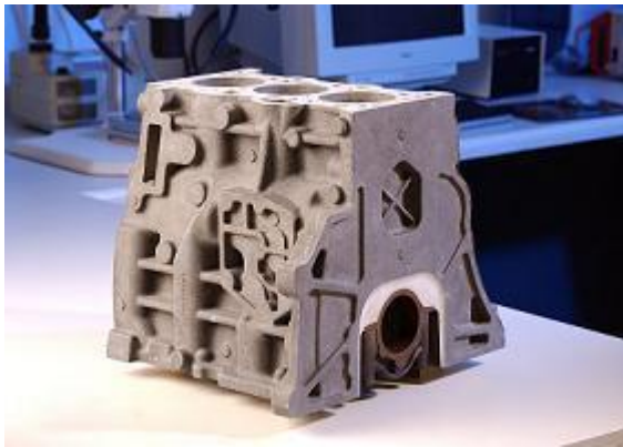
Figure 5-10: 14 kg engine block made from AM-SC1 magnesium alloy. (Source: The Engineer, 2005)
