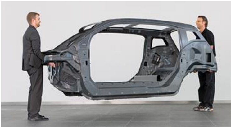
Figure 5-6: CFRP upper body structure of the 2013 BMW i3
