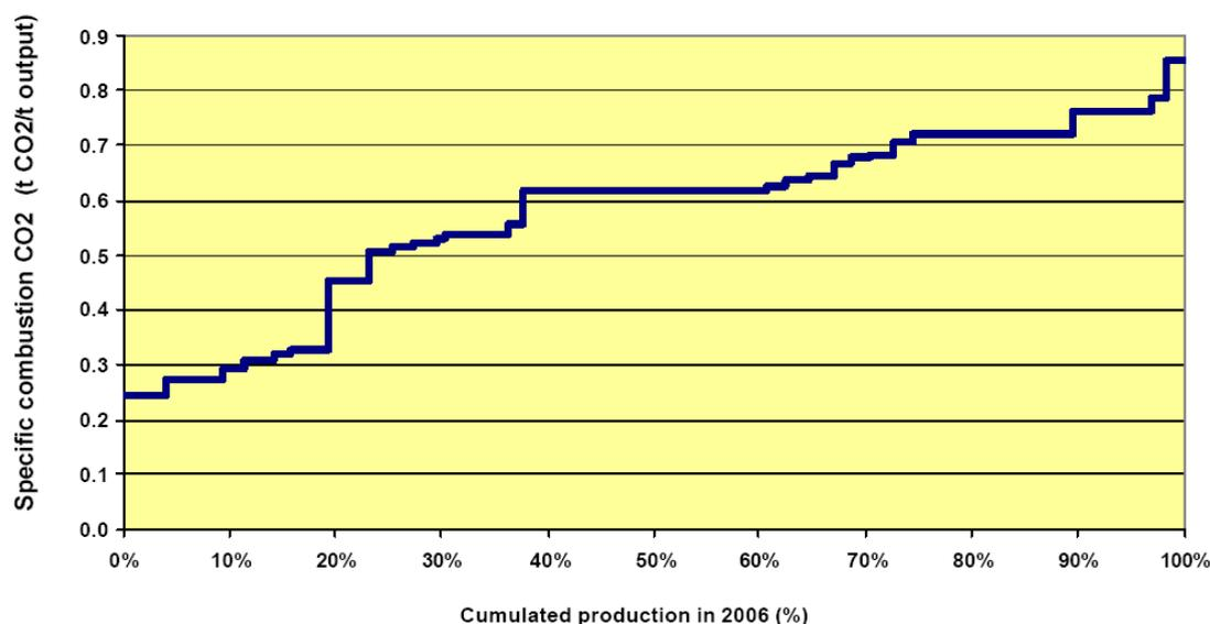
Figure 4 Specific combustion CO<sub>2</sub> emissions versus cumulated production for horizontal kilns (CIBA, 2007)
