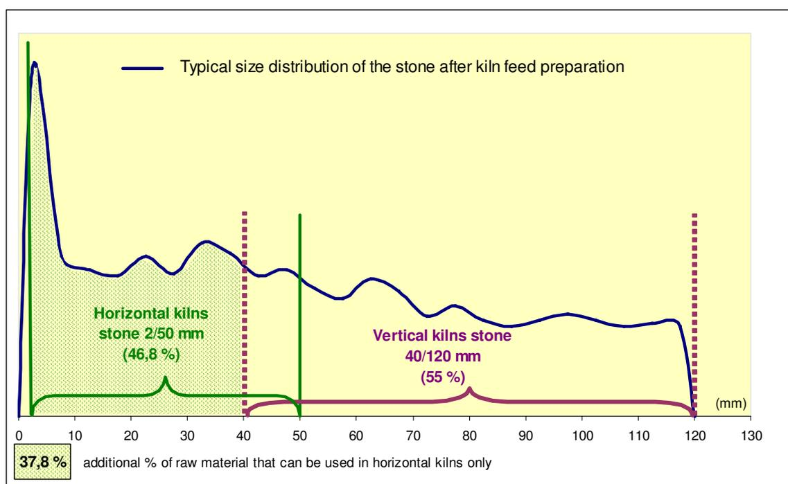
Figure 2 Typical size distribution of the stone after kiln feed preparation
