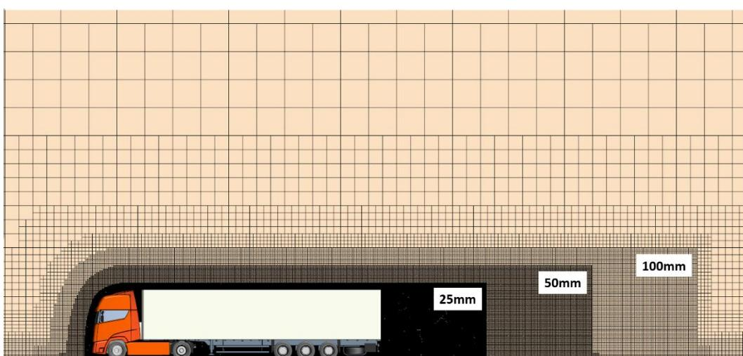
Figure 6. XZ plane section detail at Y=0
