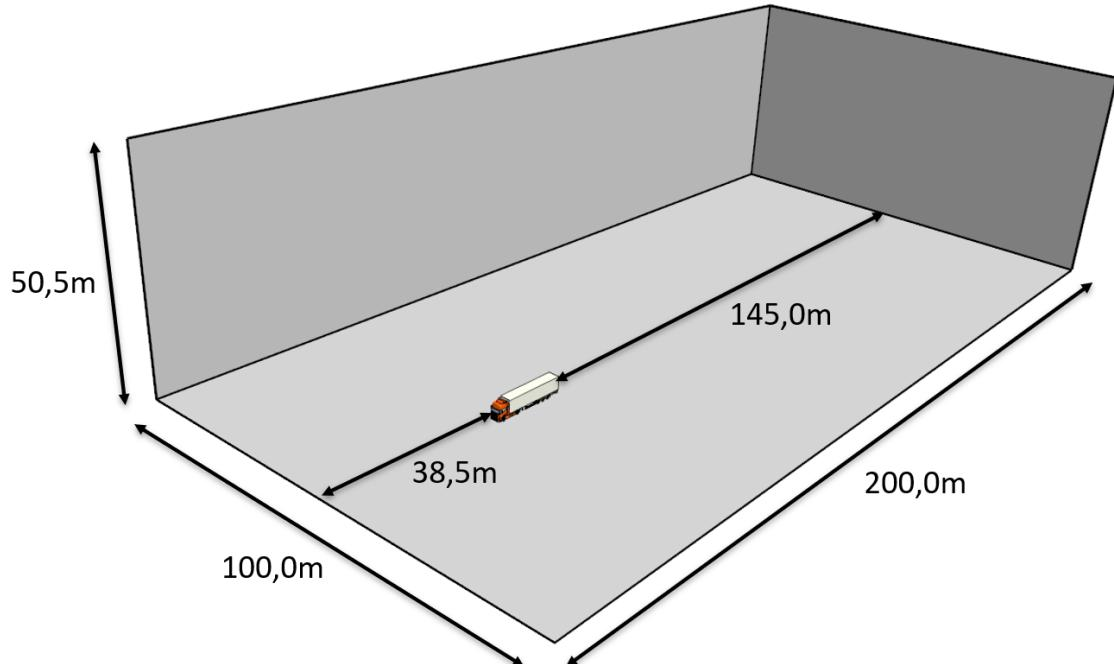
Figure 3. General domain dimensions and vehicle positioning
