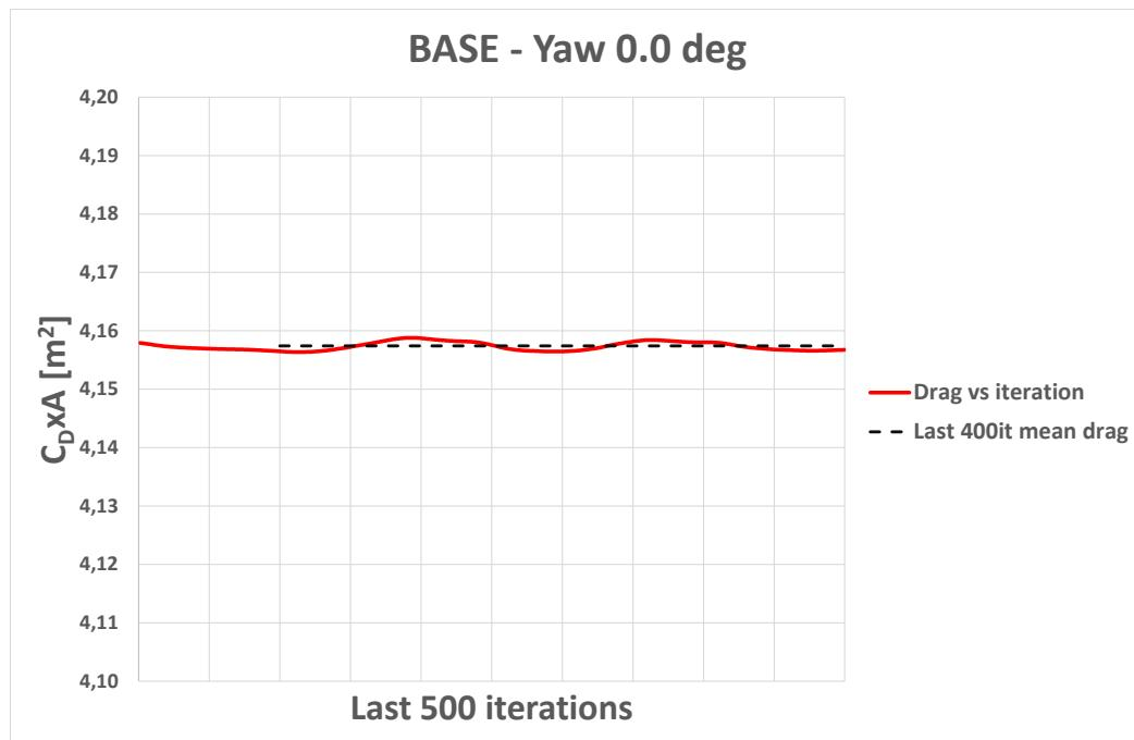
Figure 12. Drag vs iteration. Base at Yaw=0.0deg
