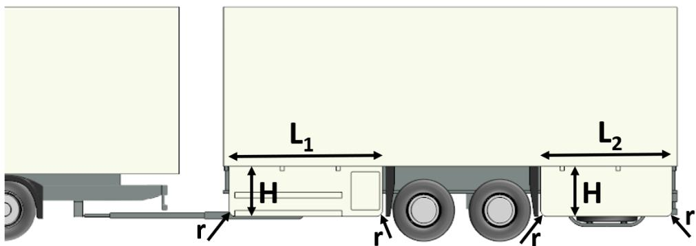
Figure 52. DC standard short side covers dimensions
