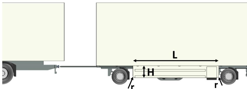
Figure 44. DB-vol standard short side covers dimensions
