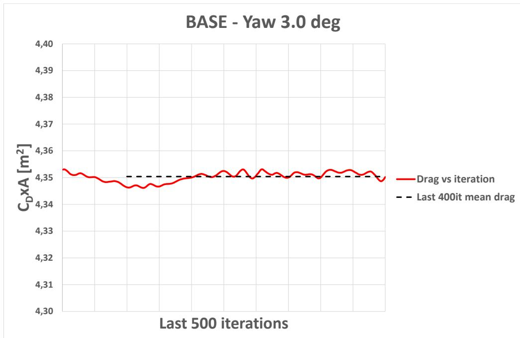
Figure 13. Drag vs iteration. Base at Yaw=3.0deg
