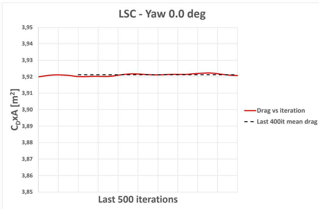
Figure 18. Drag vs iteration. LSC at Yaw=0.0deg
