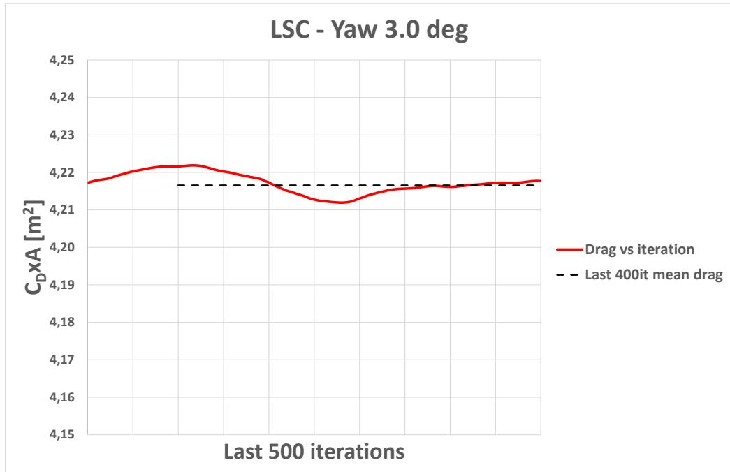
Figure 19. Drag vs iteration. LSC at Yaw=3.0deg
