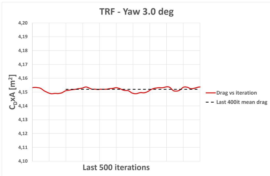
Figure 16. Drag vs iteration. TRF at Yaw=3.0deg
