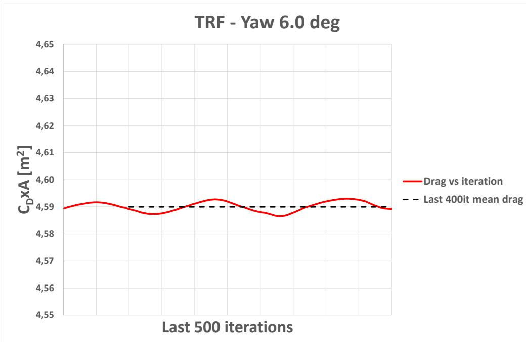
Figure 17. Drag vs iteration. TRF at Yaw=6.0deg
