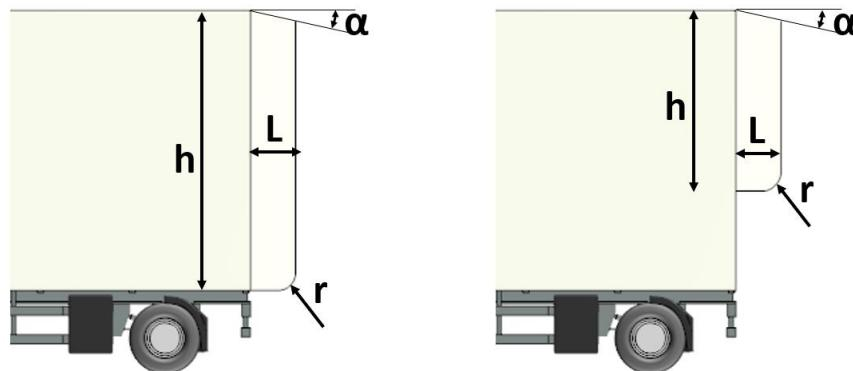
Figure 43. DB-vol standard rear flaps dimensions. TRF (left) and SRF (right)
