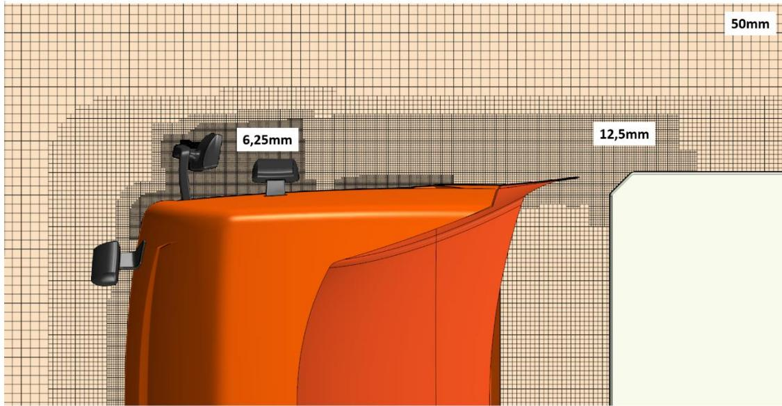
Figure 7. XY plane section detail at Z=1820mm
