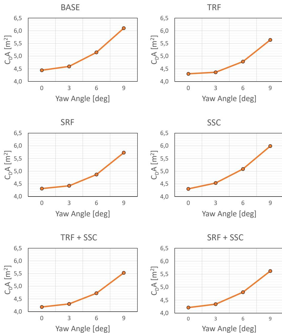
Figure 68. DB-vol. Predicted  $C_{DxA}$  [ $m^2$ ] values
