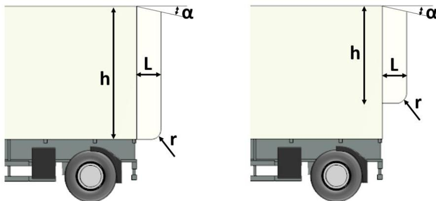
Figure 35. DB standard rear flaps dimensions. TRF (left) and SRF (right)
