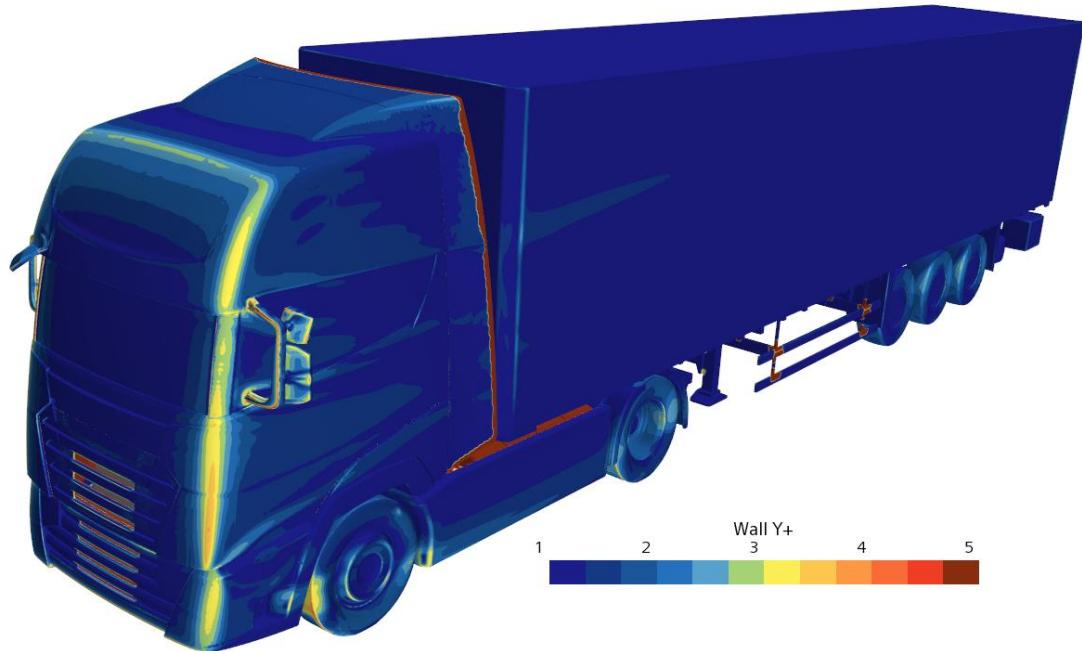
Figure 10. Wall Y+ values over the vehicle surfaces
