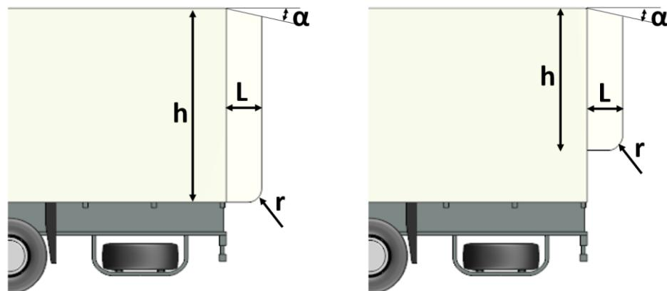
Figure 51. DC standard rear flaps dimensions
