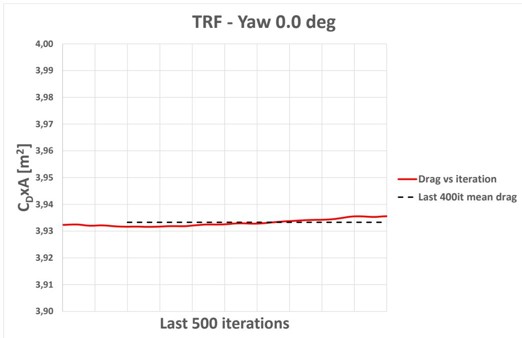
Figure 15. Drag vs iteration. TRF at Yaw=0.0deg
