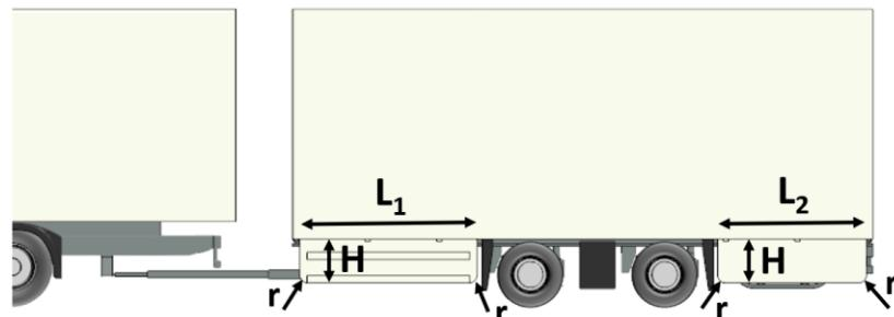
Figure 60. DC-vol standard short side covers dimensions
