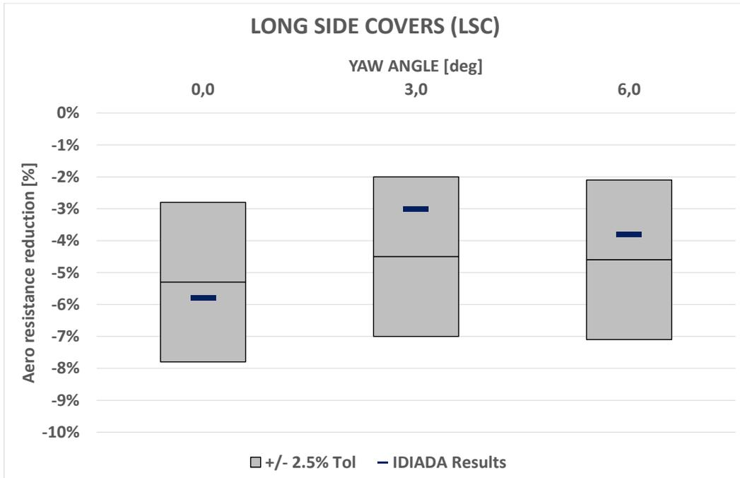
Figure 22. LSC predicted results within expected tolerance
