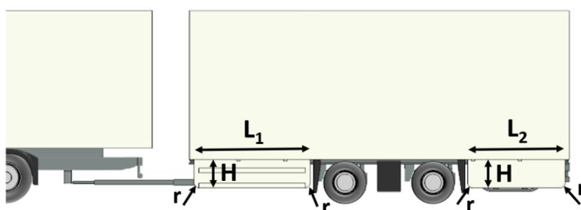
Figure 60. DC-vol standard short side covers dimensions
