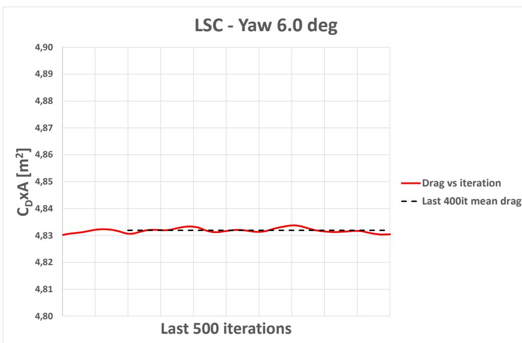
Figure 20. Drag vs iteration. LSC at Yaw=6.0deg
