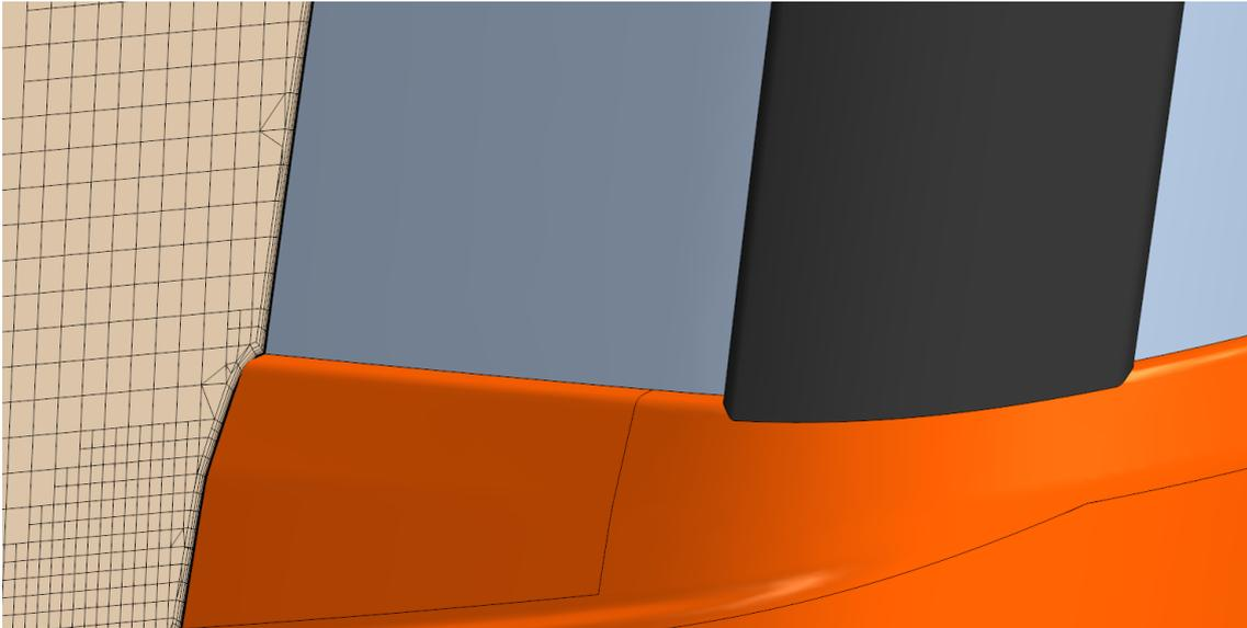
Figure 9. Prism layer detail at the base of the windshield
