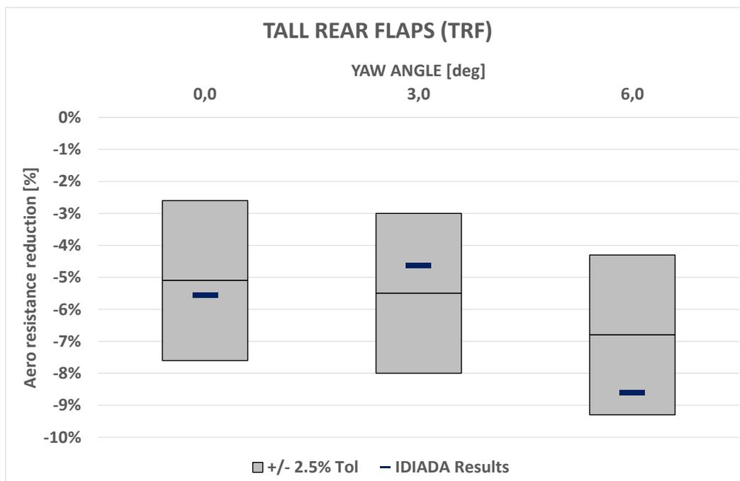
Figure 21. TRF predicted results within expected tolerance
