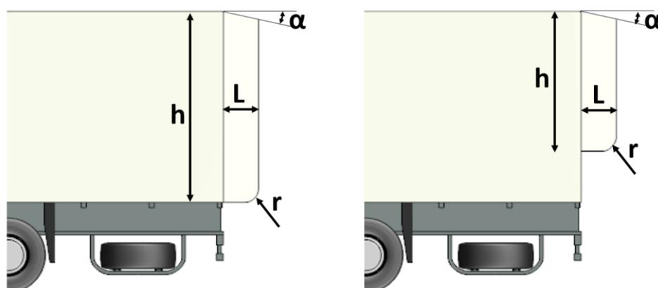
Figure 51. DC standard rear flaps dimensions
