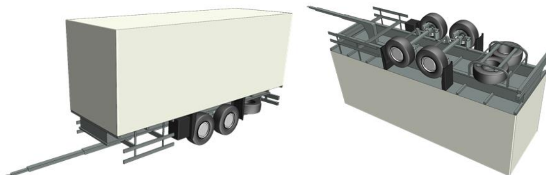
Figure 34. Standard Centre-axle trailer (isometric views)
