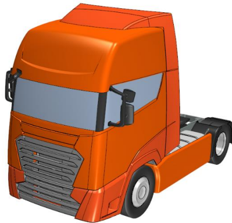
Figure 16. Isometric view of the 4x2 generic tractor model
