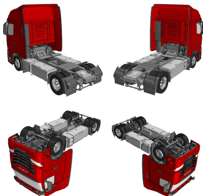
Figure 2. CAD model of the tractor IVECO Stralis Hi-Way 2019
