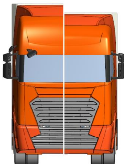
Figure 55. ST1 (left) vs Modification H01 (right). Front View
