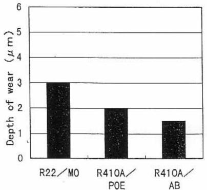
Wear depth of shaft after flooded-start test of rotary compressor
