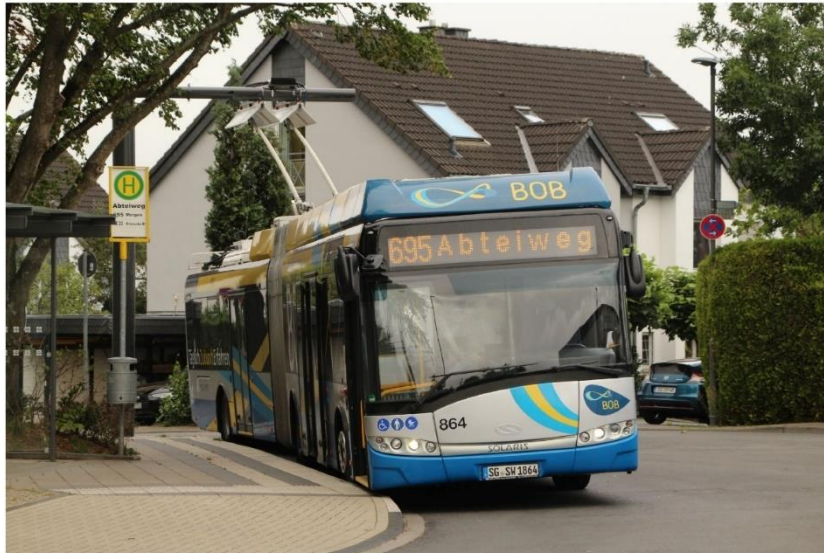
Figure 91 Trolleybus charging with Type 2 ACD at a bus stop when away from overhead lines
