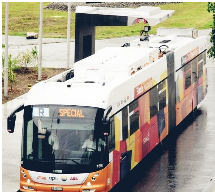
Figure 88 Laser guided connector connecting to flash charging infrastructure
