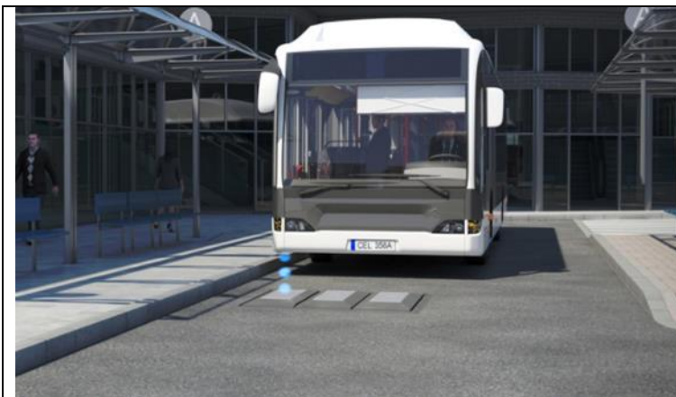
Figure 82: Floor mounted ACD Alstom solution
