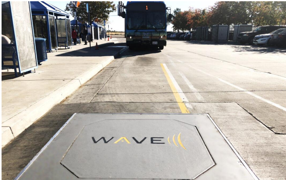
Figure 89 WAVE IPT wireless charger at a bus stop in Salt Lake City, Utah, USA [45]
