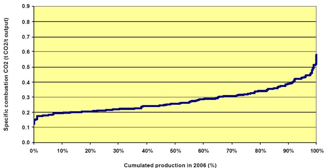
Figure 3 Specific combustion CO<sub>2</sub> emissions versus cumulated production for vertical kilns (CIBA, 2007)
