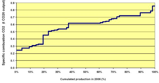
Below in Figure 4 the specific combustion  $CO_2$  emissions versus cumulated production for horizontal kilns are shown.
