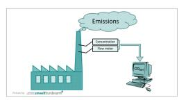
**Continuous emission measurement systems** (CEMS)
