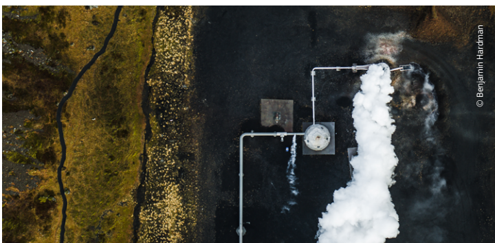
CO 2 dissolved in water is injected into underground basalt rock formations
