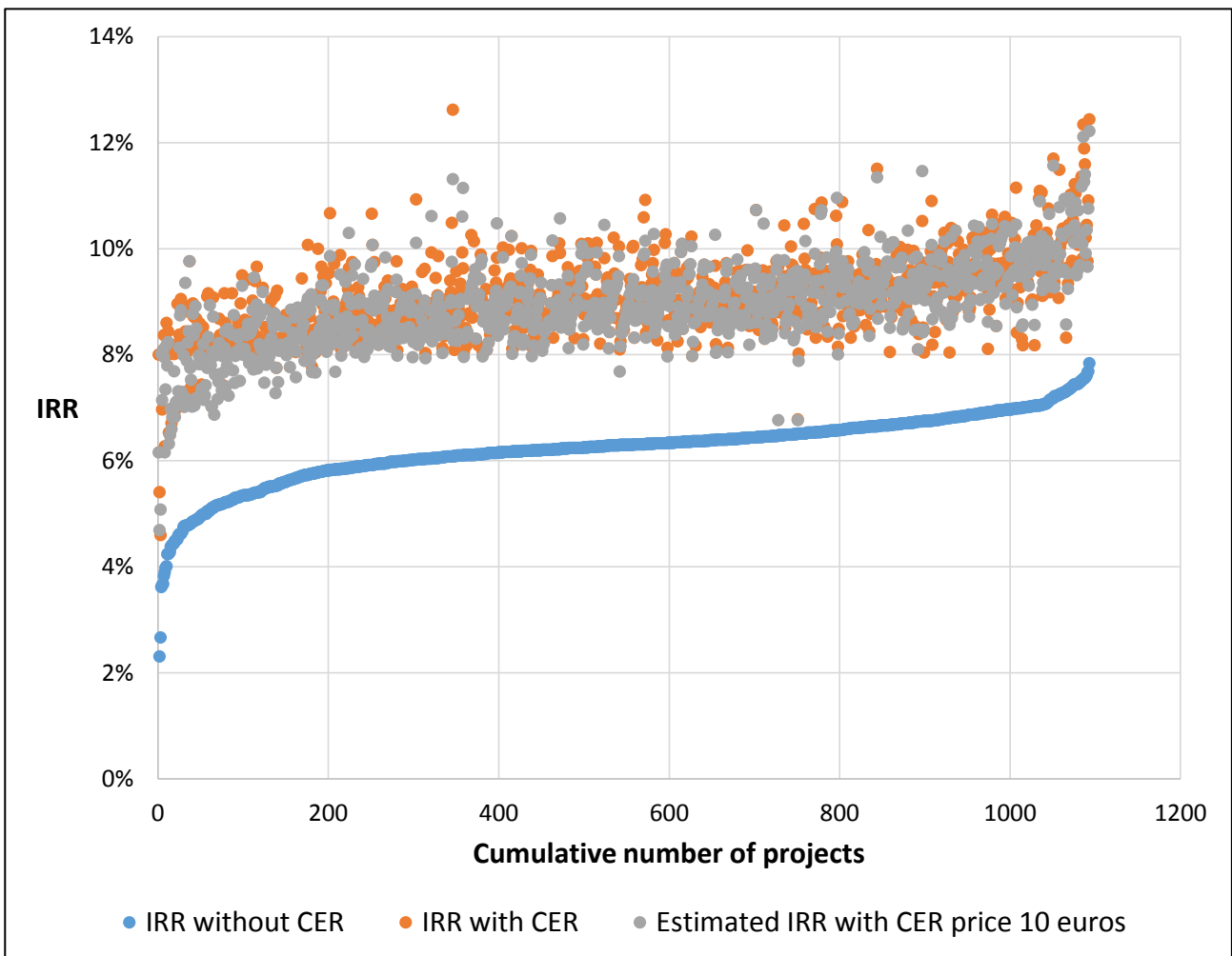
Figure 3-4: Estimated IRRs of Chinese wind projects using a benchmark of 8% before and after CER value of €10
