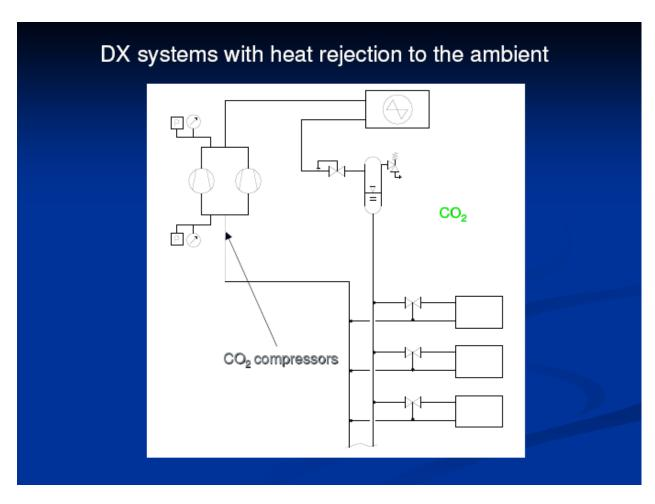
**Direct heat rejection**. It is possible to use 2 separate plants both working with CO2 as a refrigerant, in this case the two systems are completely independent and heat can be rejected directly to outside air, exactly like with conventional Direct Expansion (DX) plants working with HFC. In this case there isn't the complexity and the cost of a secondary system.
