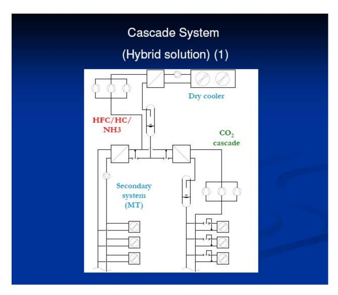
**Cascade system**. All supermarkets have two temperature levels (chilled food at 0°C and frozen food at -30°C) a first possibility is to use a conventional systems, charged with common refrigerants HFC (in some cases NH3 – Ammonia) for the cabinets / cold rooms at 0°C, cooled with a secondary fluid, and at the same time using part of refrigeration at 0°C to remove heat from condenser of a LT system using CO2 as a working fluid in direct expansion
