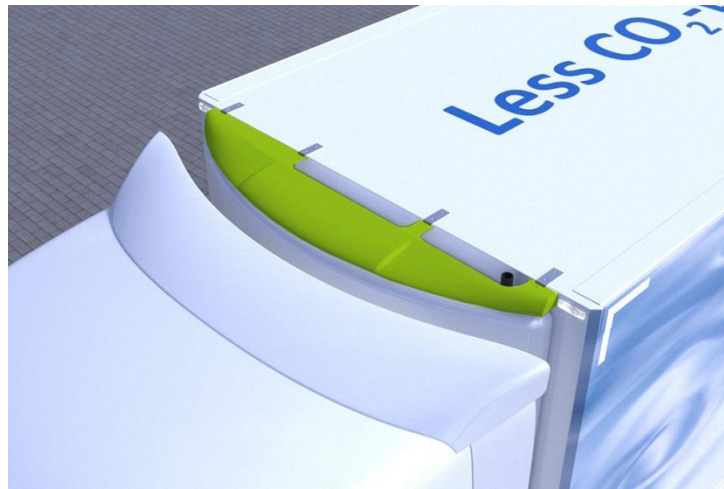
Figure 29: Example of a leading edge
