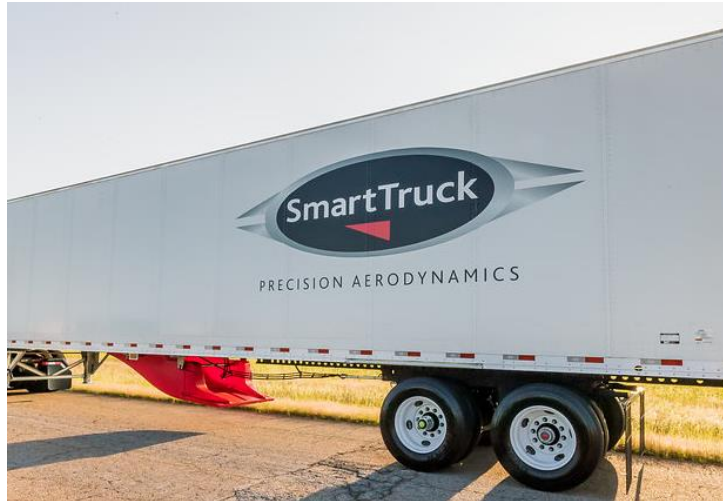
Figure 30: Example of an underbody deflector
