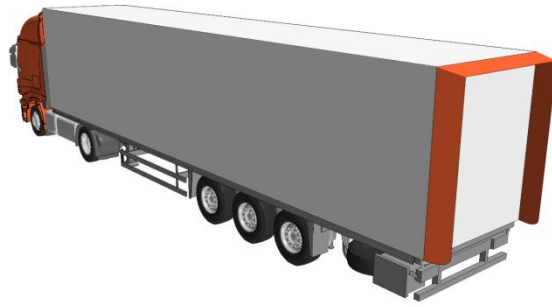
C01 – Standard semitrailer with Boat Tail
