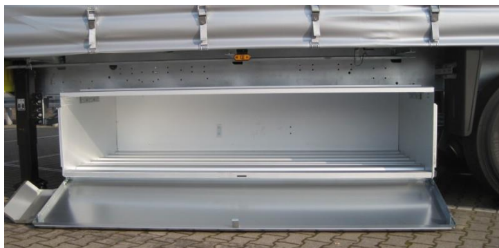
Figure 16: Example of a closed pallet box
