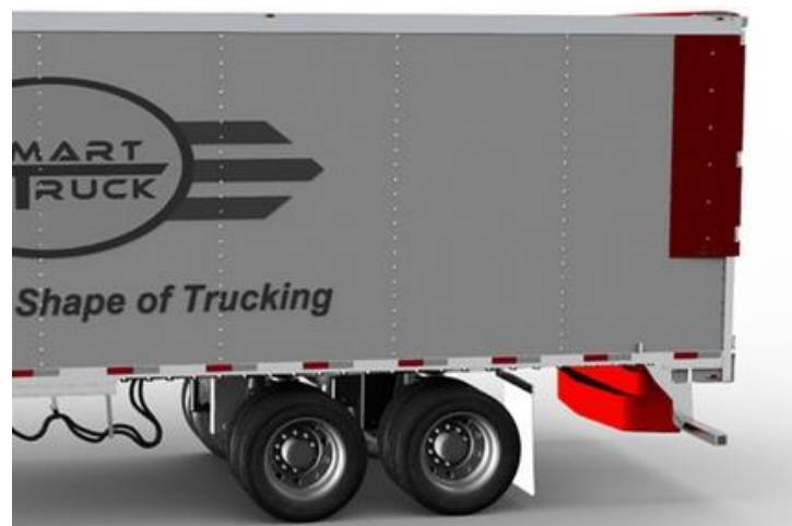
Figure 31: Example of a rear diffuser installed on a trailer
