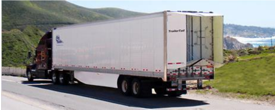
Figure 22: Example of a trailer equipped with a foldable boat tail
