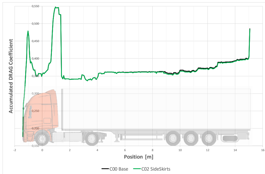
Figure 25. Accumulated Drag Coefficient. C00 vs C02. Steady-state results
