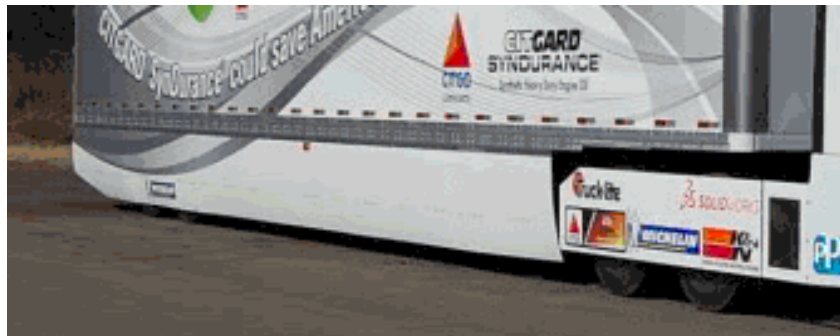
Figure 25: Example of a covered wheels full side skirt
