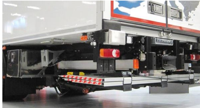
Figure 19: Example of a slider lift folded under the chassis
