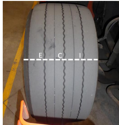
Pic. 2.- Transversal marks for tire tread depth measurement
