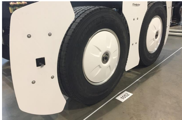
Figure 28: Example of wheel covers installed in a tractor
