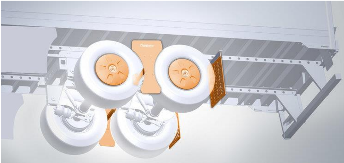
Figure 17. Wheel covers and inter-wheel panel of FlowBelow [29]
