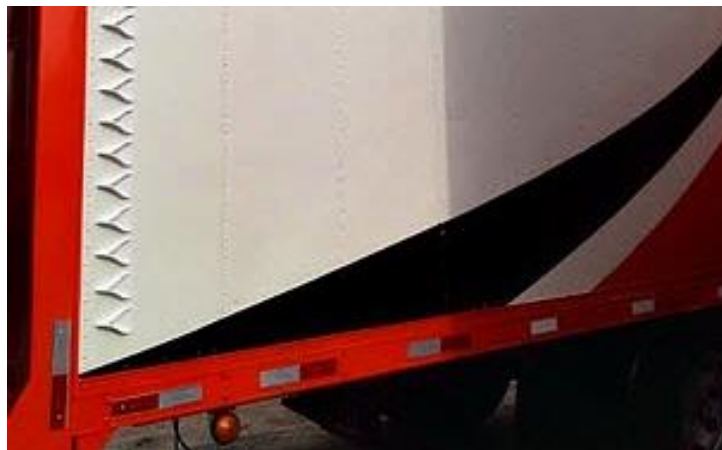
Figure 23: Example of a vortex generator system
