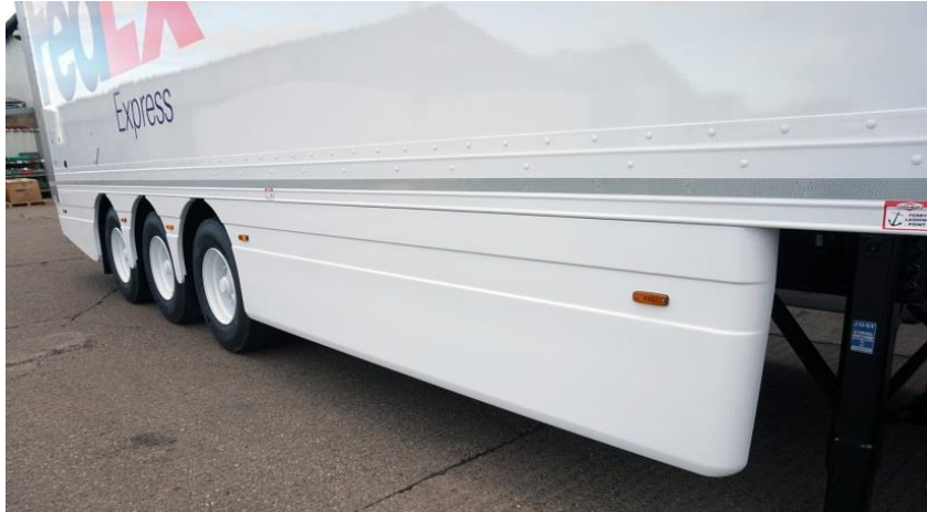
Figure 26: Example of an open-wheel full side skirt
