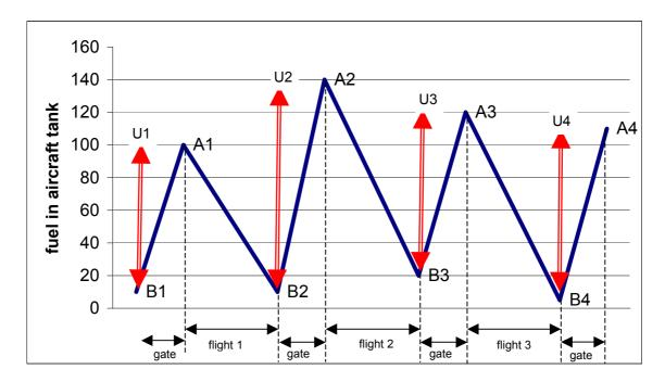
This figure represents the changes in the fuel in the aircraft tank and highlights which measurements have to be taken for calculating fuel consumption with method A or B. Measurements "A" are taken after the fuel uplift. Measurements "B" are taken on block-on at the end of the previous flight or engine shut down.
