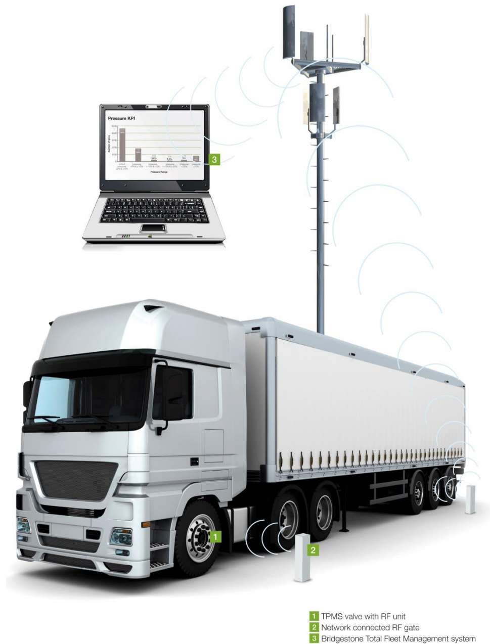
Figure 53: Bridgestone TPMS with Tyrematics [BS, 2013]
