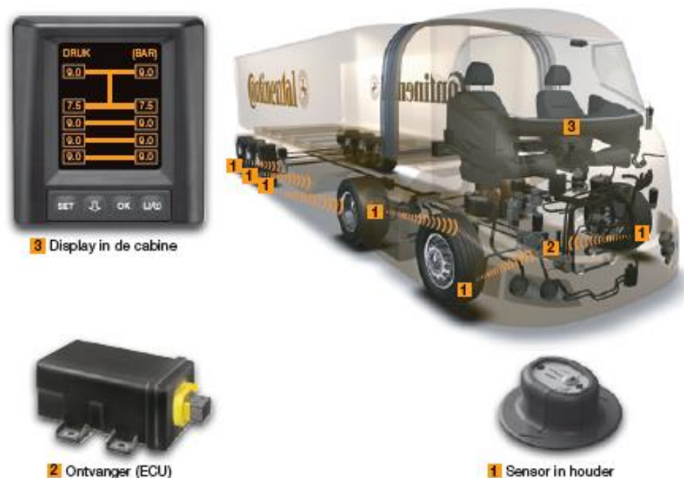
Figure 56: Continental ContiPressureCheck (CPC) [Conti, 2013]
