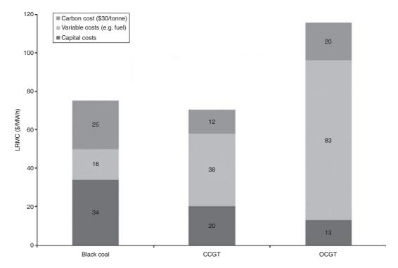
Figure 3. Long-run Marginal Cost of Thermal Technologies
