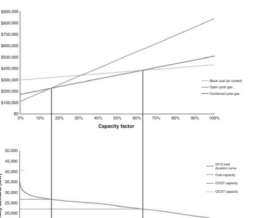
Figure 4. Optimal Plant Mix in 2010
