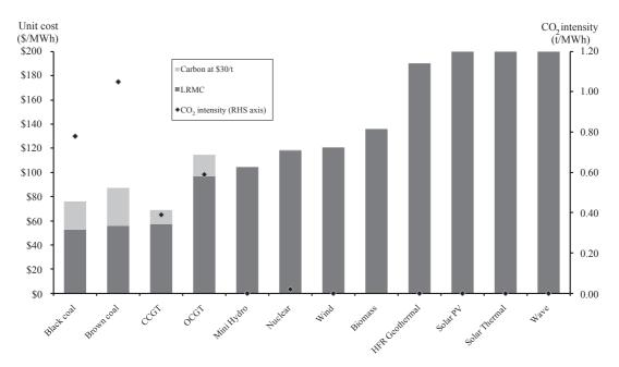
Figure 1. Long-run Marginal Cost of Power Generation Technologies
