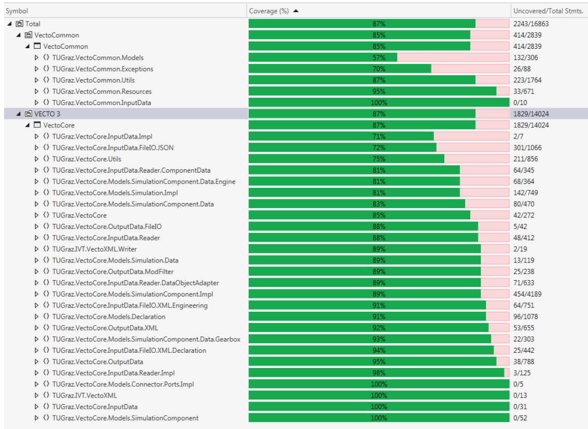
Figure 11: Test coverage measured with ReSharper
