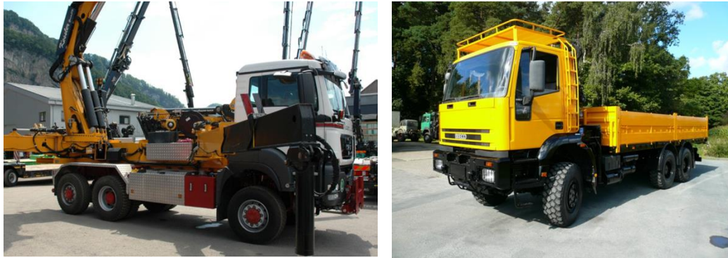
Figure 52: Example for a 6x6 rigid trucks (source www. Ditzj.de - MAN TGS 6x6 – Kessler and Hemro-Tech GmbH)
