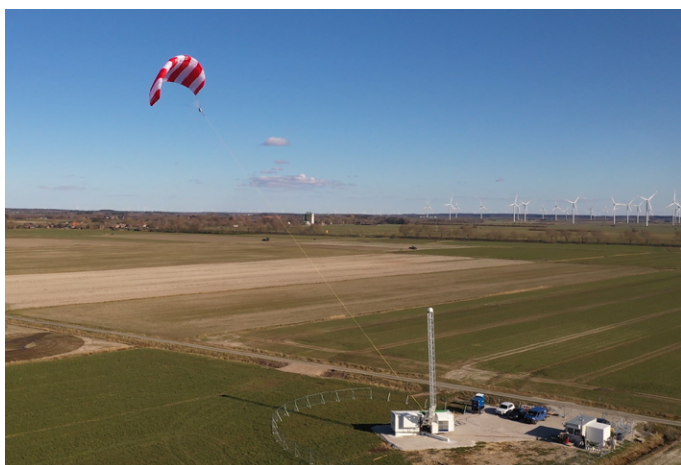
Airborne wind energy system harvesting wind speed in high altitude to produce renewable power.
