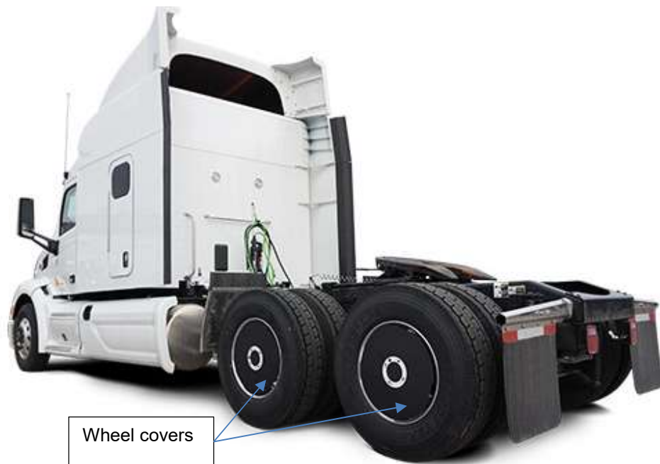
Figure 42: Example for rear truck wheels (source: realwheels.com).
