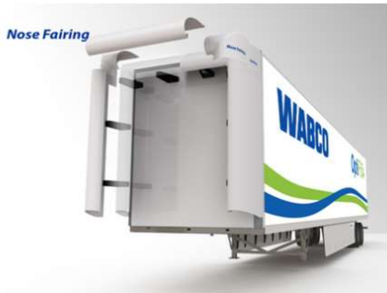
Figure 48: Rounded front edges for trailer (source: wabco-optiflow.com).
