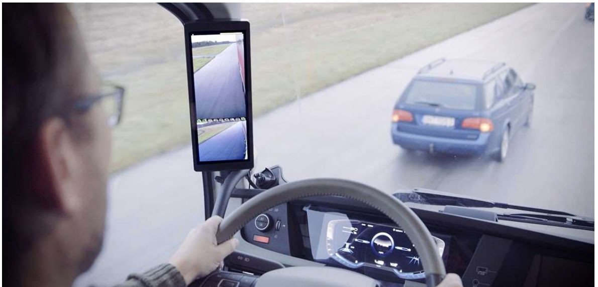
Figure 45: Rear view cameras (source: orlaco.de).
