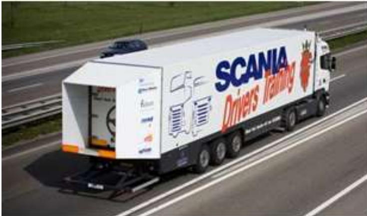
Figure 50: Boat tail application on a tractor trailer (source: part20.eu).
