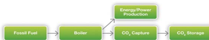
Figure 2.2 Post-combustion capture of CO 2
