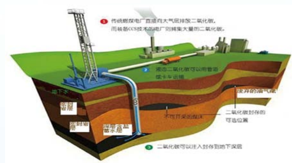
Figure 2.1 Schematic diagram of CCS system (Image courtesy of Shell; text modified by AEA)
