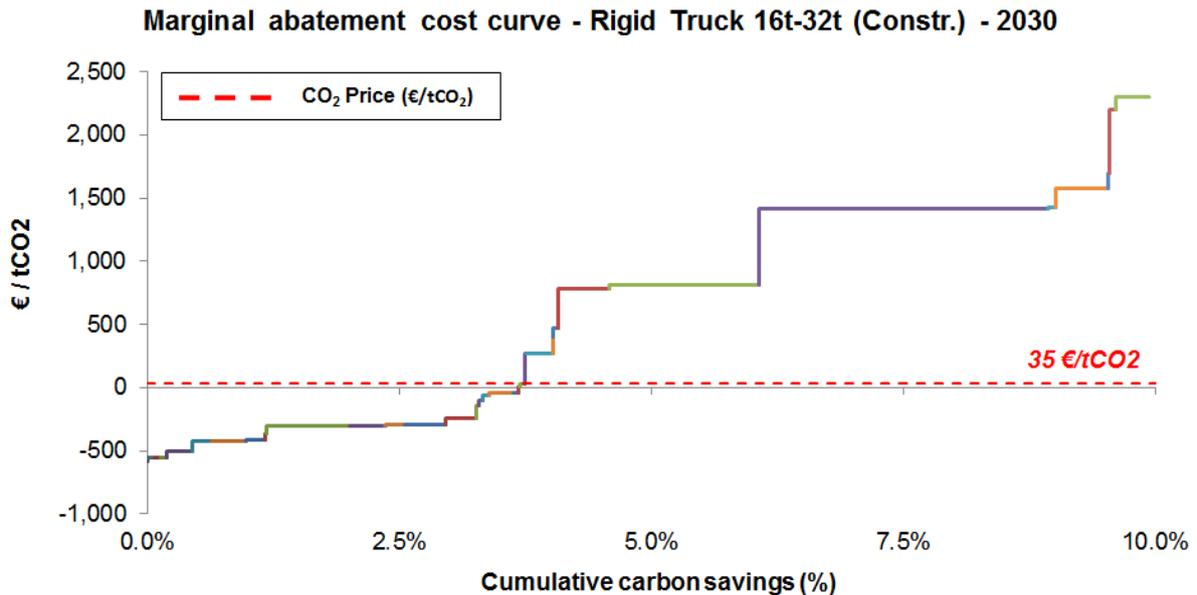
The situation is also similar with respect to CO<sub>2</sub> savings: construction trucks have the greatest cost-effective potential of all truck duty cycles. Almost 3.7% cost-effective weight reduction may be achievable by 2030 and 5% by 2050. These figures are substantially greater than those of the other truck duty cycles; one of the principal factors contributing to this is their greater levels of weight-limited operation.
