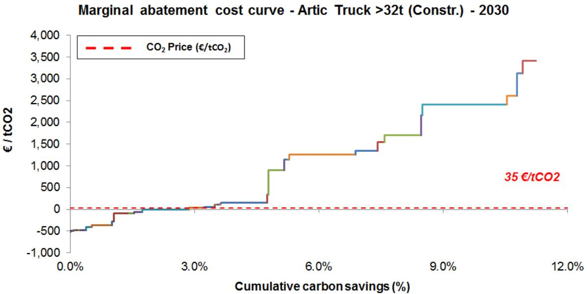
Figure 4.18: Marginal abatement cost curves for >32 tonne truck over the construction cycle (high average % weight limited operation)
