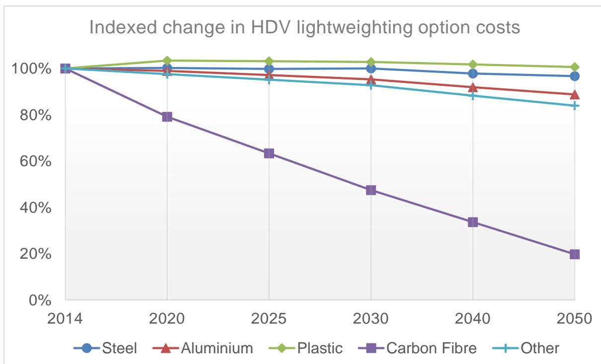
Notes: Projected increases in costs for steel, aluminium and plastic are driven by a combination of increased energy costs for the production process and increased raw material costs. Estimated improvements through learning/cost reductions for the processing of raw materials into finished HDV components is also included.
