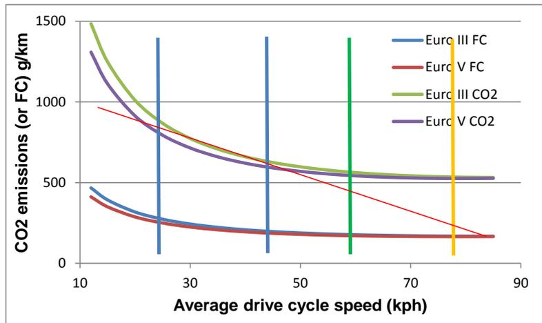
Note: blue vertical lines denote 25 and 46 kph (for phase 1 and 2 of RWUTC) green vertical line is at 59 kph, average speed for VECTO regional delivery cycle, and yellow line is at 75 kph, average speed for VECTO long haul cycle
