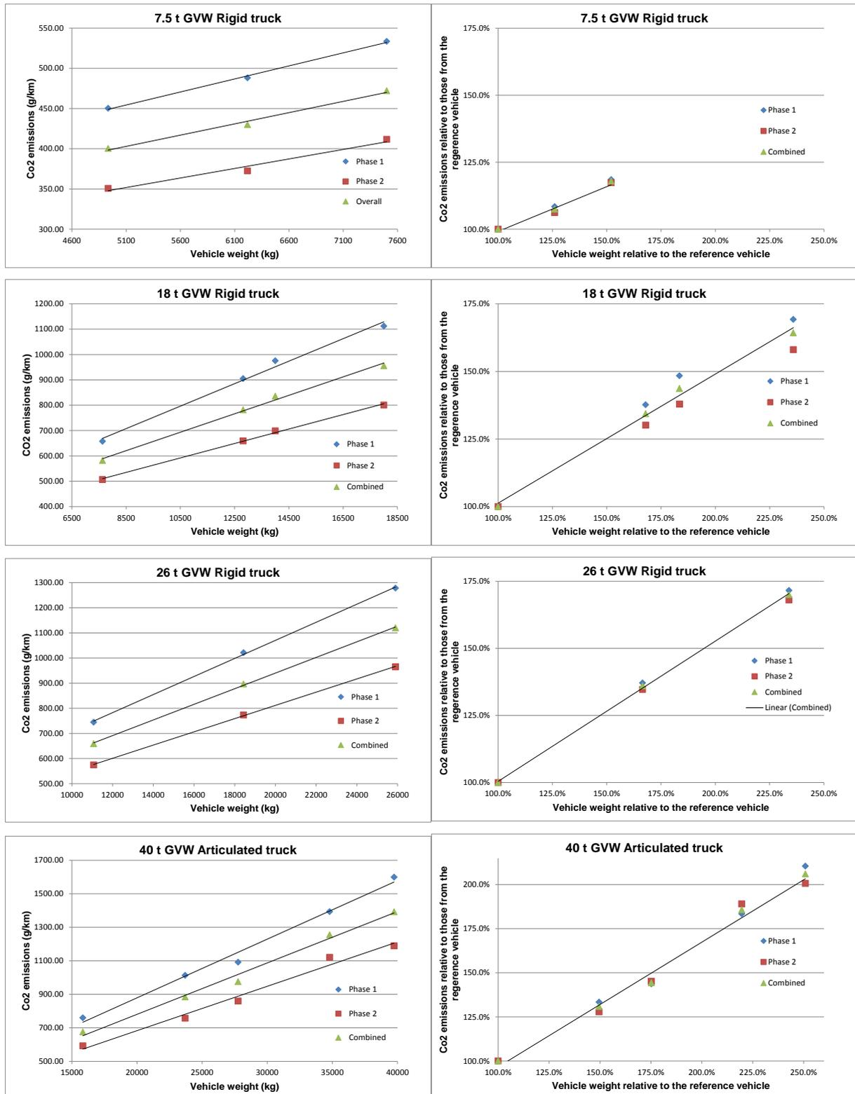
As for the VECTO simulations, all four trucks show a linear relationship between changes in emissions, for graphs of both absolute CO<sub>2</sub> emissions against vehicle weight, and when plotted relative to the reference vehicle. Each figure also includes one least squares regression fit to emphasise this.
