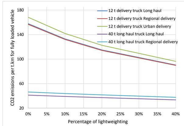
Table 3.7 tabulates the data from the linear regressions for the six vehicle type/drive cycle combinations shown in Table 3.4 and the figures above when the data are plotted as CO<sub>2</sub> emissions against vehicle weight. The table also contains the R<sup>2</sup> value for the regression. This is always equal to, or greater than, 0.9996, i.e. the correlations are all very close to linear
