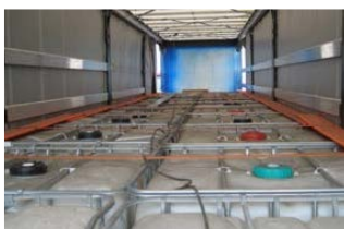
Figure 38: Water tanks in the trailer of HDV 4
