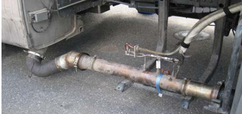
Figure 39: Semtech Exhaust Flow Meter connected to the tailpipe
