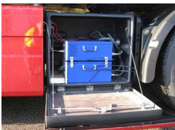
Figure 40: Example of installation of KMA Mobile in a heavy duty vehicle
