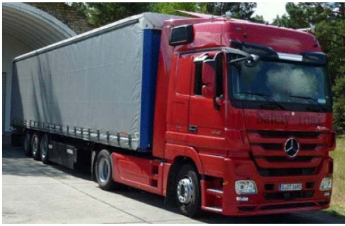
Figure 86: Articulated truck with a gross vehicle weight of 40tons (“HDV4”)
