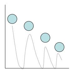
The same way a rubber ball does not rebound as high as it was launched, energy is dissipated when a tyre rolls and is deformed.
