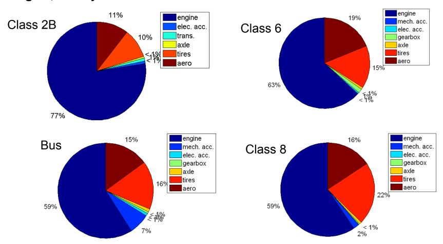
Vehicles at GVWR and 50 mph Steady State Speed
