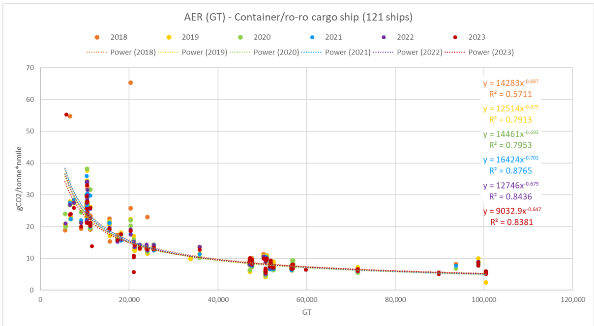
Figure 40: Plot of attained AER values of container-ro-ro cargo ships over the reporting years and associated trendlines
