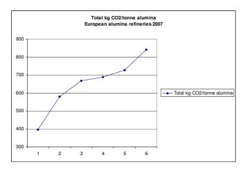
Figure 1 Preliminary benchmark curve on alumina production, 2007 (EAA, 2009)
