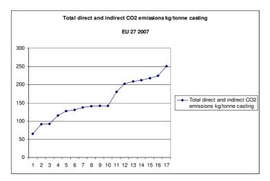
Figure 4 Preliminary benchmark curve on primary casting without remelting, including indirect emissions, 2007<sup>14</sup> (EAA, 2009)
