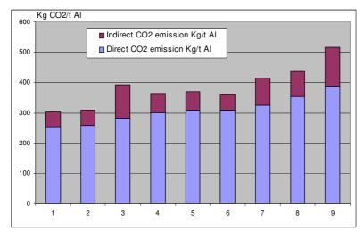
Figure 7 Preliminary benchmark curve on secondary aluminium (refining) including indirect emissions, 2007<sup>14</sup> (EAA, 2009)
