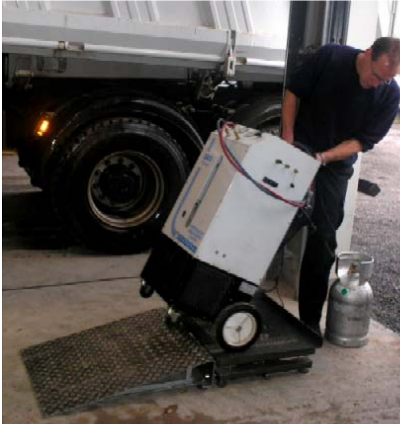
Figure 10: Service station Waeco RHS 650 on the scale after the recovery operation.
