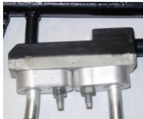
Photo 1.5 – Details of the inlet and the outlet fittings of the condenser
