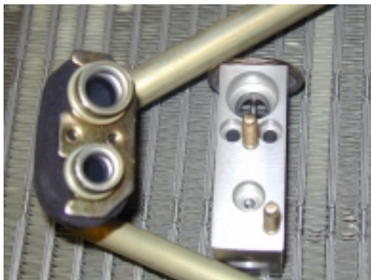
Photo 1.4 – Details of inlet and outlet fittings of the evaporator to be fitted in the expansion valve
