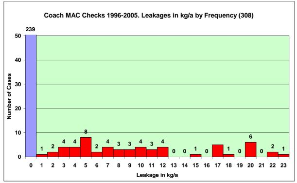
Diagram 4: The average annual MAC leakage rate of the coach sample of 1.50 kg/a is an arithmetic figure which consists in reality of a large number of "zero-leaks" and a smaller number of highly diverse actual leaks varying from <1 to more than 20 kg/a.
