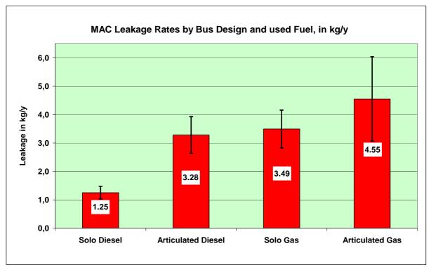
Diagram 2: Bus MAC leakage rates widely vary by vehicle design (solo or articulated) and by fuel type (diesel or gas). Solo diesel buses show the lowest values with 1.25 kg/a. This is a statistically significant difference from the other vehicles (no overlapping error bars).
