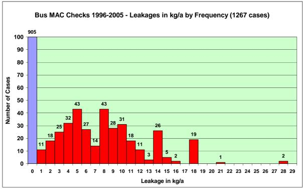
Diagram 1: The MAC leakage rate 2.34 kg/a of the bus sample is a computed figure which consists in reality of a large number of "zero-leaks" (blue bar) and a smaller number of highly diverse actual leaks (refills) varying from 1 to more than 18 kg/a (red bars).
