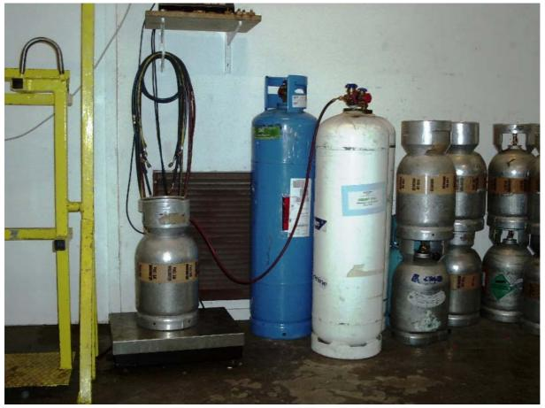
Kylindustri garage. Before refilling, refrigerant HFC-134a is decanted from a 60-kg container into a portable 10-kg cylinder which is weighed out on the scale.
