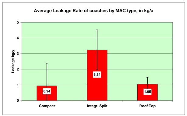
Diagram 5. Leakage rates of coaches widely vary by MAC design. Integrated split systems show a significantly higher average value with 3.24 kg/a compared to only 1.05 kg/a of roof top systems (no overlapping error bars). Compact systems, which show a numerically low leakage rate of 0.94 kg/a only, are too small in number for meaningful statistical analysis.
