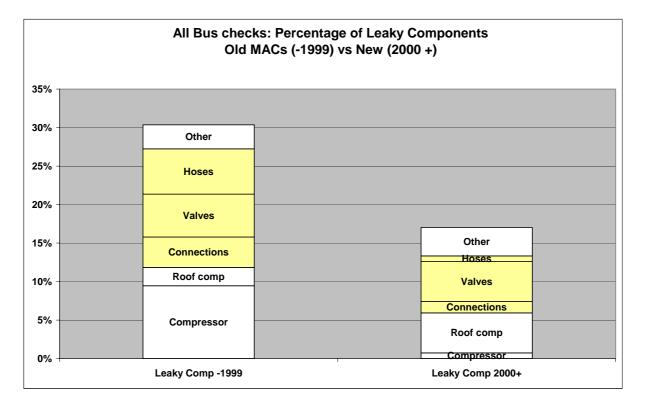
Both Table 26 and Diagram 8 show marked differences between older and newer MAC systems. (It should be realised that the percentage shares of the components do not add up to 100% but to 100% minus the shares of "zero leaks").
