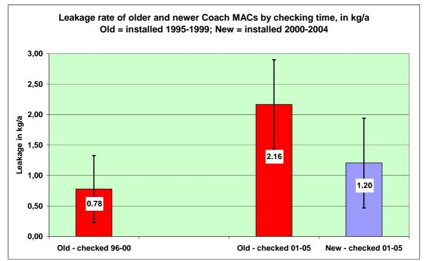
Diagram 6: Visible small spaces between the error bars of the leakage rates of the two old age-classes (red) prove that the differences between old coaches, checked 1996-2000, and old coaches, checked 2001-2005, are statistically significant, indicating the so-called ageing effect. The nominal leakage rate of 1.20 kg/a of new coaches checked 2001-2005 (blue) is not lower but higher than that of old systems, checked the first five years from installation.
