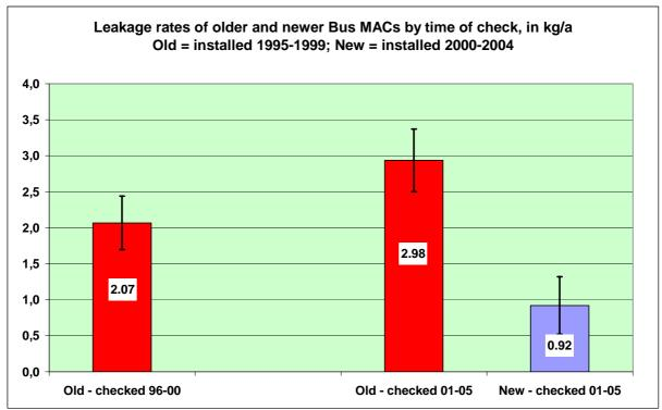
Diagram 3: Visible spaces between the error bars of the annual leakage rates of the three bus age-classes indicate that the differences between old buses, checked 1996-2000, and old buses, checked 2001-2005, are statistically significant; this also applies to the low leakage rate of new buses from 2000 onwards (checked 2001-2005) with just 0.92 kg/a.
