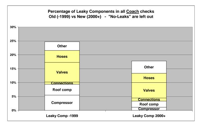
Both Table 28 and the Diagram show results of interest. (It should be realised that the percentage shares of the components do not add up to 100% but to 100% minus the shares of "zero leaks").
