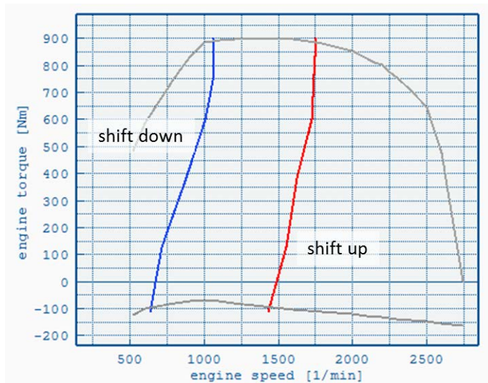
Figure 74: Example of up- and down- shift curves for VECTO's gear shift model
