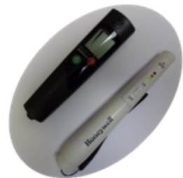
Figure 2, flammable gas detectors
