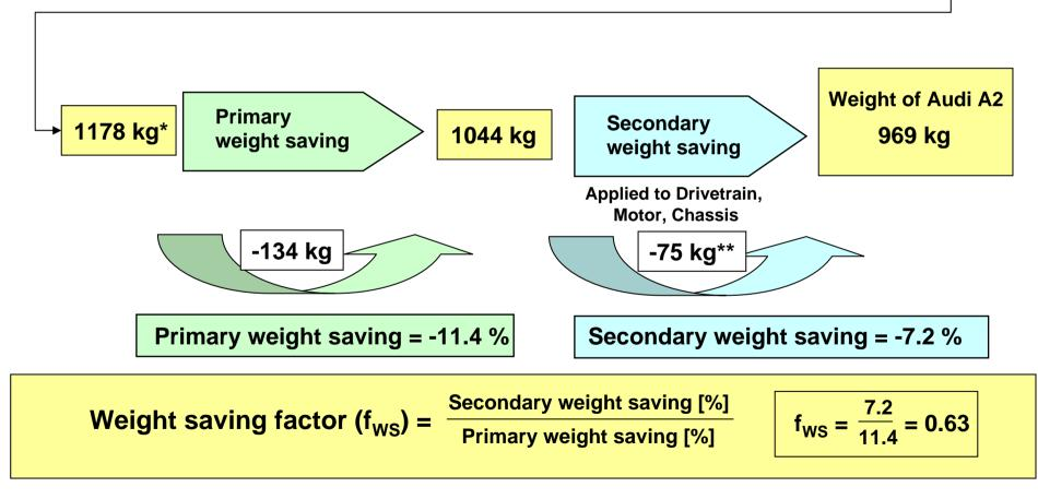
\* adjusted for 42 kg fuel weight / \*\* adjusted for 21 kg fuel + tank weight
