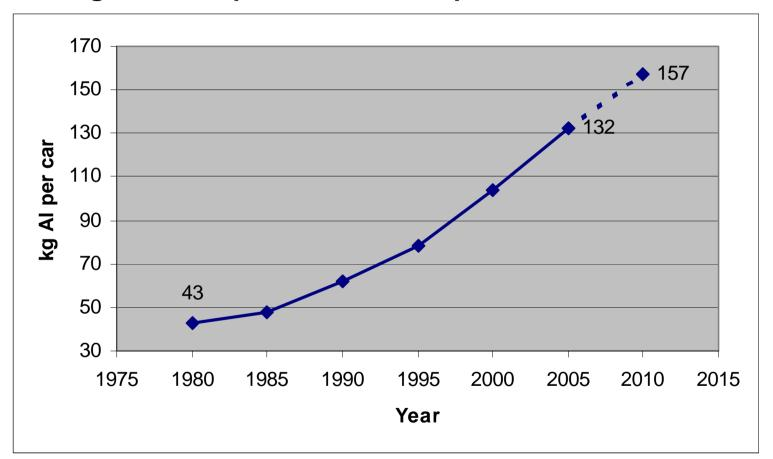
The Audi A2 contains more than 300 kg of aluminium The Audi A8 contains about 520 kg of aluminium alu)
