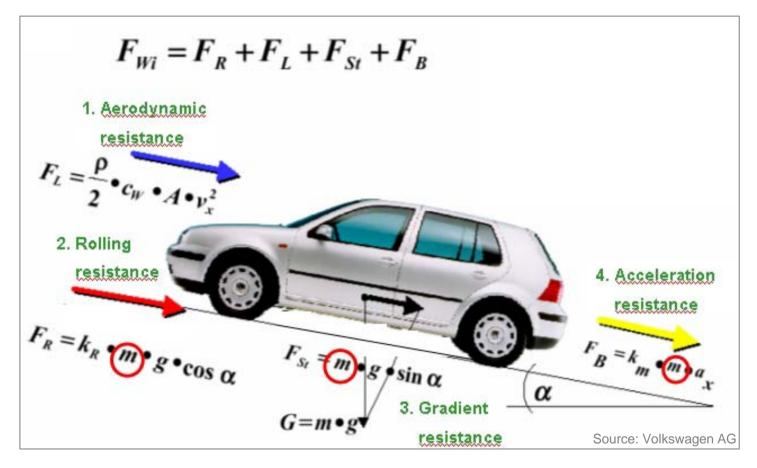
The energy required to move a vehicle is, except for aerodynamic resistance, directly proportional to its mass
