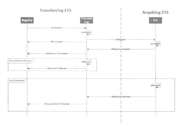
This reflects the point of view of the transferring ETS. The sequence diagram above depicts all the specific outgoing transaction flows.
