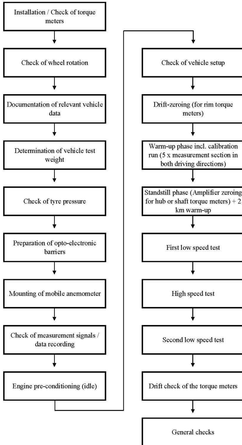
**Fig. 5-1: Constant speed test**
