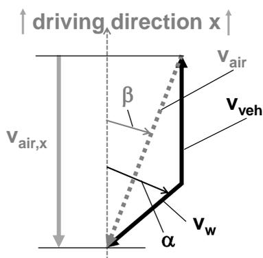
**Fig. 5-1: Geometrics of air flow and vehicle speed**
