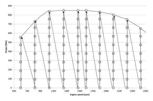
Fig. 5-2: Measurement points for fuel map
