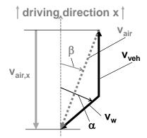
Fig. 5-1: Geometrics of air flow and vehicle speed
