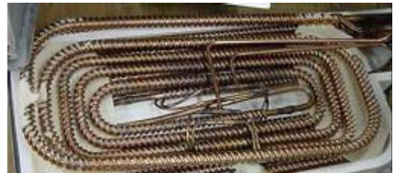
Photo of appearance of water heat exchanger
